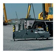
**Removable outrigger boxes** Removable front and rear outrigger boxes provide up to 8788 kg (19,374 lb) of weight reduction for easier transport. Includes the removable 18 100 kg (40,000 lb) of counterweight, auxiliary hoist and rope, and the RT9130E-2 can easily self-remove close to 29 000 kg (64,000 lb).
